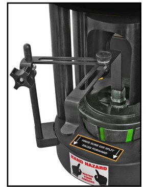
Adjustable coupling stop for accurate, repetitive positioning of the assembly inside the dies
