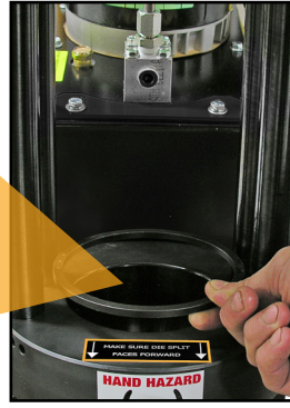
Matched die and spacer crimp eliminates need to adjust settings
