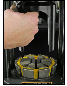
Removable pusher and rubber cage die sets for easy loading
